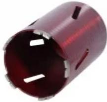
A premium dry core bit with spiral barrel design for swift dust removal. Features include a fast start segment, side vents and a spiral barrel design to help keep the bits cool resulting in longer life. Suitable for use in masonry, brick, concrete with light or medium steel reinforcing. Also effective for granite, marble and stone.
