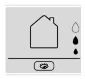
Surveillance Mode in the AUREN 160 Single-Room Heat Recovery Ventilation Unit is a standby feature designed to monitor humidity levels and activate extraction only when necessary. It operates silently with the front panel closed until humidity exceeds a set threshold, at which point it switches to extraction mode at medium or night speed, depending on the time of day.
