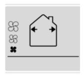
The AUREN Extract Only Mode is a specialised function that allows the unit to operate solely in extraction mode, removing stale air from a room without supplying fresh air. This mode is particularly useful for quickly eliminating excess humidity, odours, or pollutants, making it ideal for kitchens, bathrooms, or other high-moisture areas.
