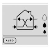
The AUREN Automatic Mode is an intelligent ventilation setting that adjusts airflow based on humidity and twilight sensors, ensuring optimal air quality and energy efficiency. During the day, it operates at medium speed with heat recovery, while at night, it switches to a lower speed for quieter operation. If humidity exceeds set thresholds, it activates extraction mode to maintain a healthy indoor environment.
